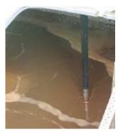
Over a period of months, the ISE measuring procedure has permanently delivered exact nitrate values in the biological cleaning.
